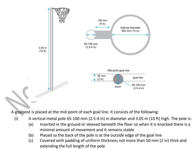
(ii) A horizontal metal ring made of steel rod 15 mm (5/8 in) in diameter with an internal diameter of 380 mm (15 in)
